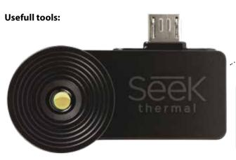
Seek Thermal is the most advanced thermal imaging camera for smartphones
