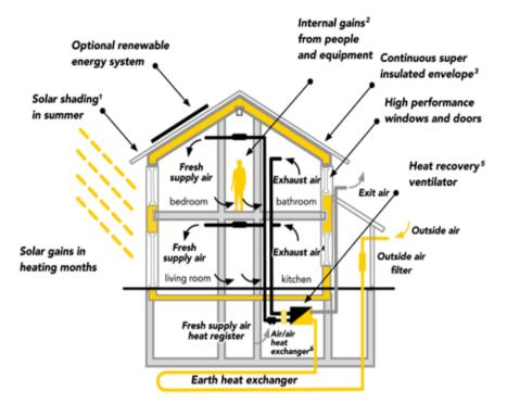
used to keep the house cool. The warmth inside or heat outside is achieved thanks to the highly insulated walls, roof, floor slab and special energy efficient windows. Ventilation supplies guality air.
