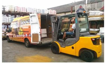
DFG 425s. The hydrostatic transmission on the DFG 430s and the automotive VW engine offered precision control and improved fuel efficiency in handling loads up to three tonnes.
