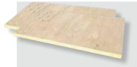
It is high performance external wall board with a fibre-free rigid thermoset phenolic core used for external insulation on masonry walls behind traditional and lightweight polymer modified renders and dry cladding systems.
